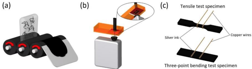
Figure 8.1. Manufacturing process of the nanocomposite specimens: (a) calendaring dispersion process, (b) DLP 3D printing process and (c) electrode placement on 3D printed specimens.
