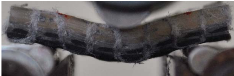
(c) Load applied on the glass face of a specimen with z-yarns. No evidence of cracks were found at this deformation level.
