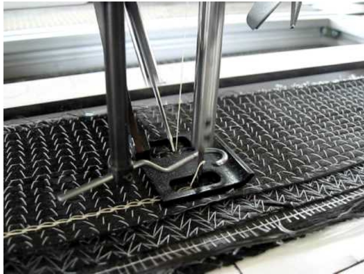
Figure 1.5: Common 3D textile techniques: weaving, warp-knitting, braiding and stitching.
