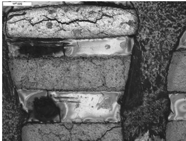
(c) Extensive cracking at carbon tow (top) caused by longitudinal shear stresses
