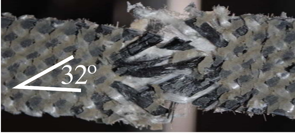
Figure 5.4: Angle between fibres measured after failure.
