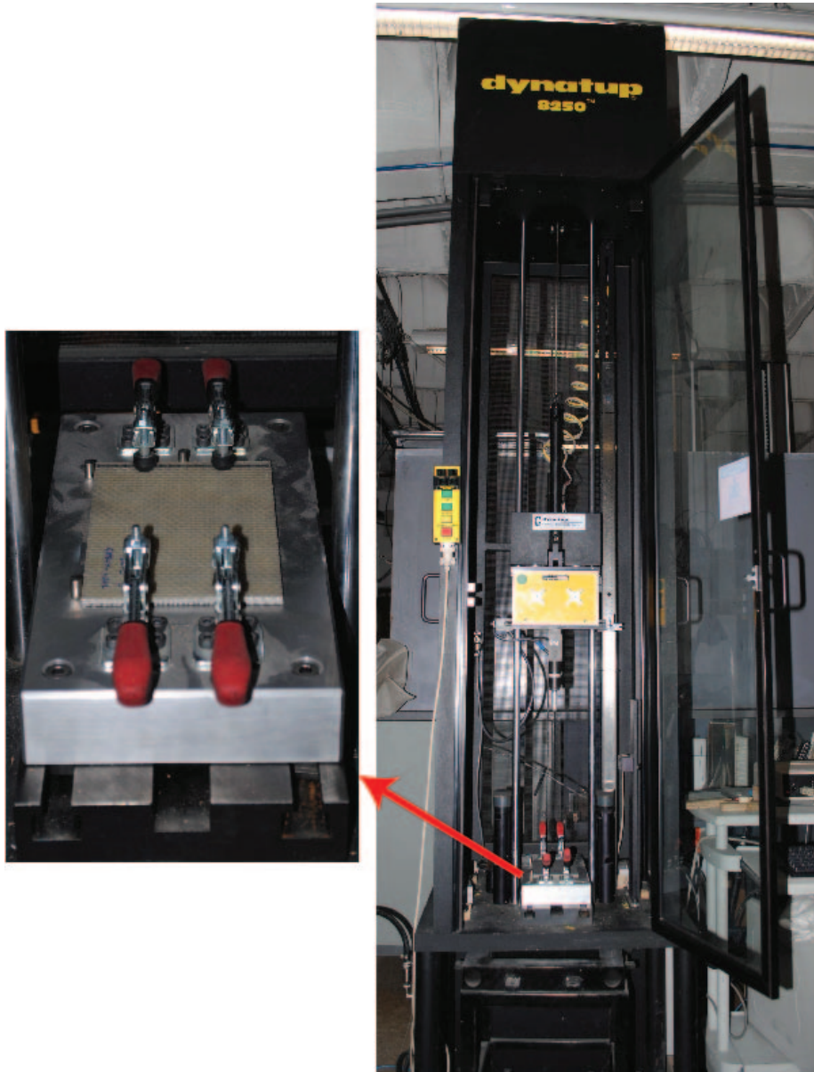
Figure 6.2: Drop-weight set-up. Detail of the coupon and the clamping tweezers.
