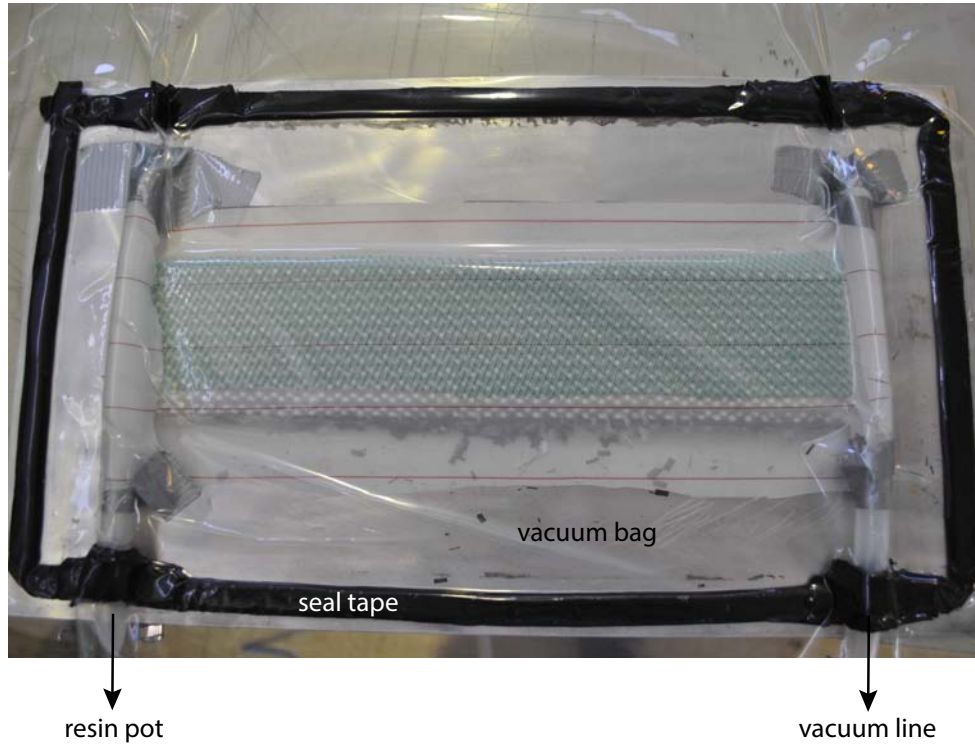
(a) Processing set-up during infusion by VARTM.
