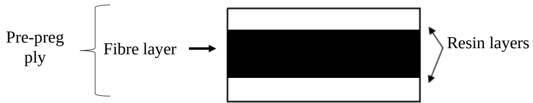
Figure 6.1. First hypothesis considered for the pre-preg modelling
