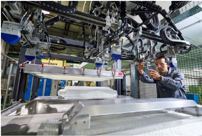
Pick & place automated cell.
